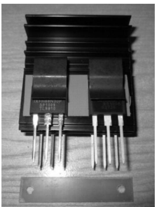
After placing all other components, it's time for the MOS-Fet transistors.
